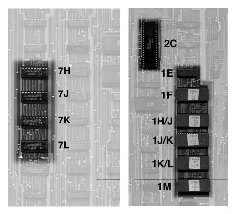
You'll be replacing the PROMs (on the left, 7H-7L); replacing the PROMs (on the right, 1F-1M); removing the NOVRAM at 1E; as well as soldering on a wire to the 6809 in location 2C and placing the daughtercard in the socket at 1H/J and 1E.
