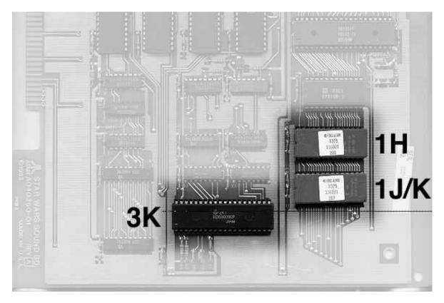
Later on you'll be soldering a wire to one of the pins of the 6809 at location "3K' and replacing the ROMs at locations "1H" and "1J/K".
