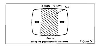
NOTE: Static convergence is achieved by four magnets located on the neck, nearest the base of the picture tube, Fig. 2. The middle pair of magnetic rings are adjusted to converge the blue and red crosshatch lines. The rear pair of convergence rings (closest to the base of the picture tube) are adjusted to converge the magenta (blue/red) to the green crosshatch lines. Dynamic convergence is achieved by tilting the deflection yoke up-down and left-right.
