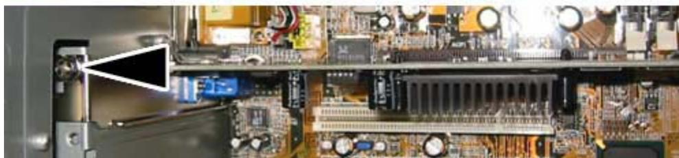
6. You need to be sure that the video card is installed correctly. Be sure there are no gold tabs showing just above the AGP slot as shown by the arrows in the picture below.
