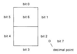
To determine what hexadecimal number to write, to the display for a given combination of segments, just set the bit, for each segment you want lit, to 1 and convert the resulting data word to hexadecimal.
