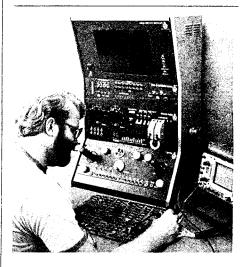
Atari's Computer Test Fixture, CTF-1, is a complete testing system for video game printed circuit boards. This is a self-contained benchtop unit designed to simulate field use of the games in a test environment. CTF-1 is the test unit that is used by factory technicians to troubleshoot all video PCBs. Field service technicians can now order this complete unit through Atari distributors.
