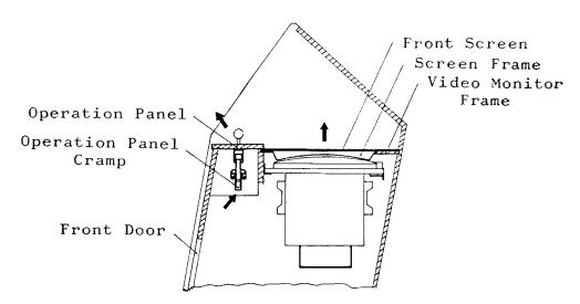
To dismount the front screen and the operation panel for maintenance of the control under or adjustment of the video monitor, open the front door and unfasten the operation panel cramp.
