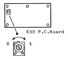
Sound volume adjustment can also be made on Video Monitor Sound P.C.Board.
