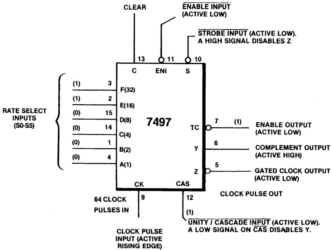
The Z output is normally high and goes low when CK and STROBE INPUT are low and any of the inputs (S0-S5) are high. The Y output is the complement of output A and is thus normally low.
