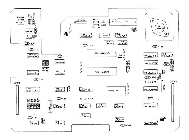
Figure 10.1 Logic Board Layout
