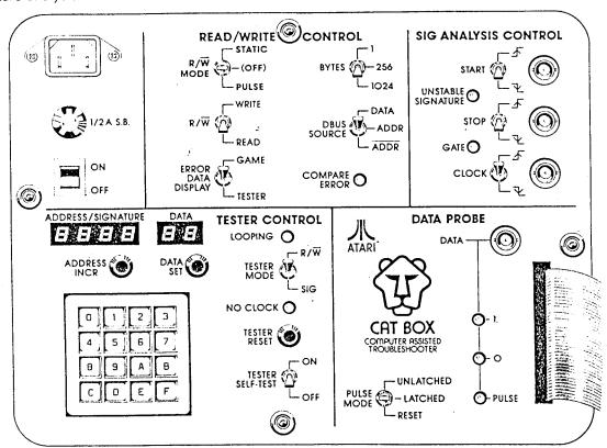
Figure 8.1 The CAT Box Control Panel
