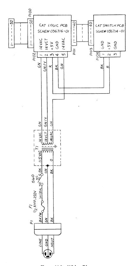
Figure 11.3 Wiring Diagram
