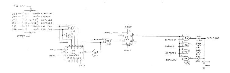
Figure 6.6 Discrete Audio Outputs (Asteroids Deluxe<sup>TM</sup>)
