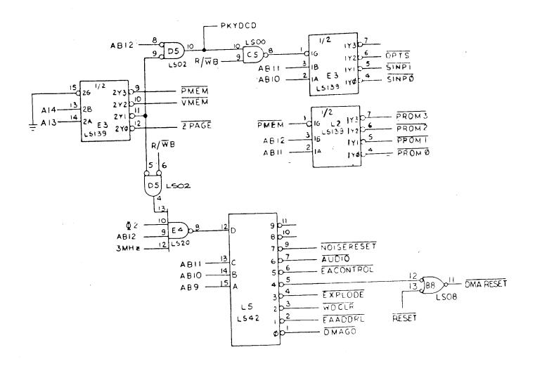
Figure 6.3 Address Decoding (Asteroids Deluxe<sup>TM</sup>)
