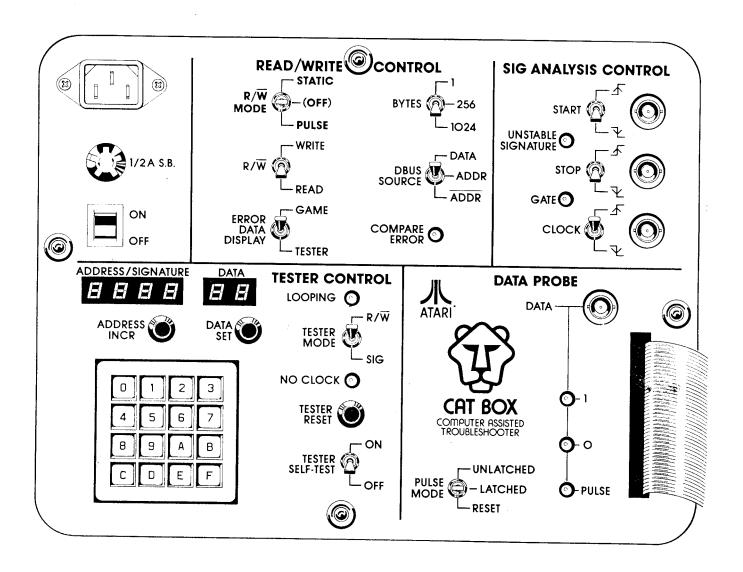
Figure 1.1 CAT Box Front Panel
