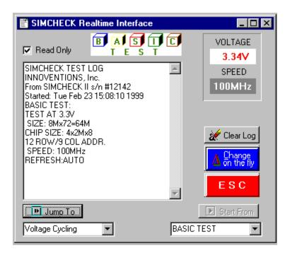
A summary of the module's size, mode type, access time, and cycle time, along with the list of the various control signals is displayed after the Basic Test. Also displayed are messages indicating if the module is nonstandard, or otherwise different in architecture.
